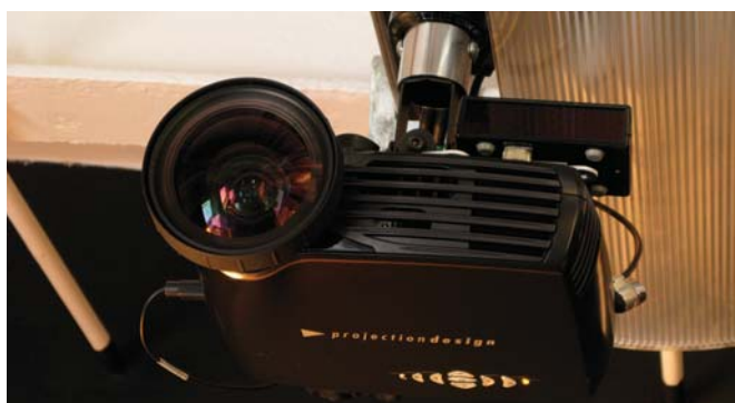
A high-performance projector sends images to the diffusion screen.
